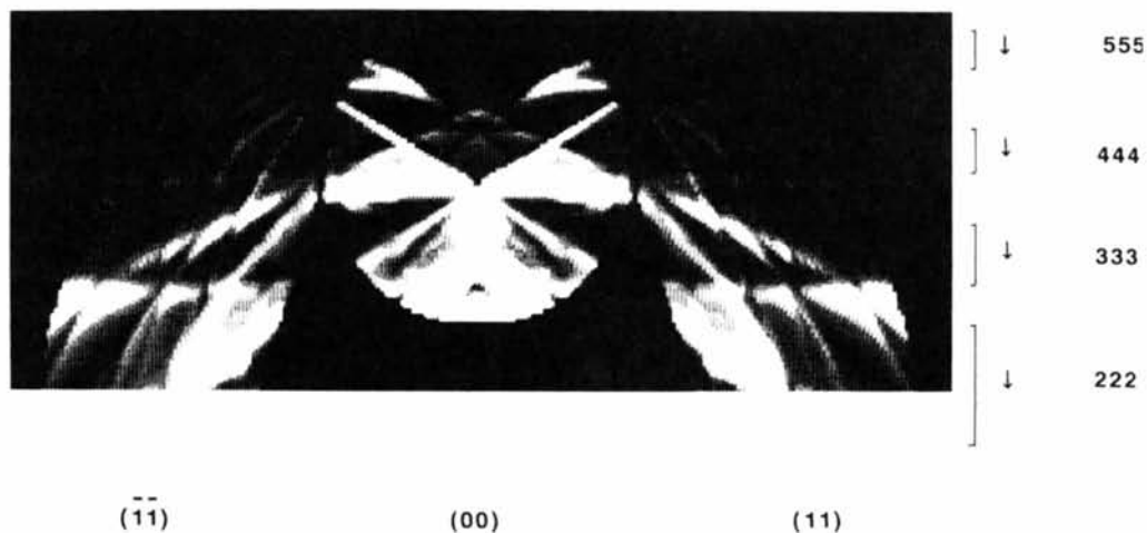
Fig. 2. Results of dynamical CB-RHEED calculations for the same parameters as in Fig. 1 but with a circular aperture in the incident beam. The colatitude angle of incidence at the centre of the circular disc defining the pattern circumference is 1.4^\circ corresponding to 5.5c^* reciprocal-lattice vectors. The central azimuthal angle is set equal to zero. The aperture radius is 0.8^\circ corresponding to one half of the reciprocal-lattice rod spacing.
